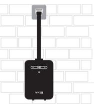
➤ The WiFi Status Light will flash blue showing it's in pairing mode. If it is not flashing blue, press and hold the left Power Button until the light begins to flash blue.
