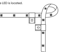
**Trimming the Strip:** The strip can be cut but only at the designated marks, as shown in the diagram below. Do not cut the strip except at a designated mark. Before cutting the strip, make sure the power adapter **is unplugged.** The trimmed portion of the strip cannot be used and
