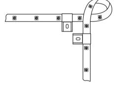
Trimming the Strip: The strip can be cut but only at the designated marks, as shown in the diagram below. Do not cut the strip except at a designated mark. Before cutting the strip, make sure the power adapter is unplugged. The trimmed portion of the strip cannot be used
