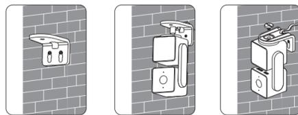
Note: When installing, make sure there's at least 30 mm clearance around and 150 mm above your mounting location. Your bracket screws should be exactly 21 mm apart.
