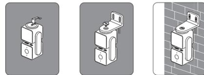
Note: When installing, make sure there's at least 30 mm clearance around and 150 mm above your mounting location. Your bracket screws should be exactly 21 mm apart.
