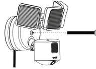
NOTE: When attaching the floodlight to the mounting plate, do not let the power cable of the floodlight rest on top of the metal sheet of the mounting plate. Ensure that the floodlight screw is tightened securely.
