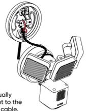
3 Connect the hot wire (usually black) from your floodlight to the hot wire from your power cable. Then connect the 2 neutral wires (usually white). Cap the wires using wire nuts and twist them 5-10 times. Gently tug on the wire nut to make sure it's securely attached.
