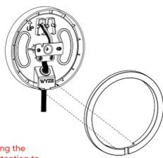
NOTE: When installing the silicone ring, pay attention to the arrow indication in the picture to ensure proper fit here.
