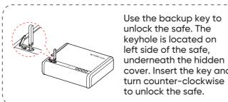
Use the backup key to unlock the safe. The kevhole is located on left side of the safe. underneath the hidden cover. Insert the key and turn counter-clockwise to unlock the safe.
