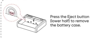
Press the Eject button (lower half) to remove the battery case.
