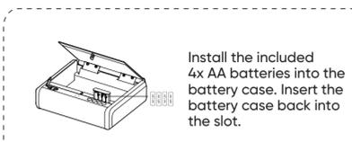
Install the included 4x AA batteries into the battery case. Insert the battery case back into the slot.
