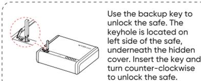
Use the backup key to unlock the safe. The keyhole is located on left side of the safe, underneath the hidden cover. Insert the key and turn counter-clockwise to unlock the safe.
